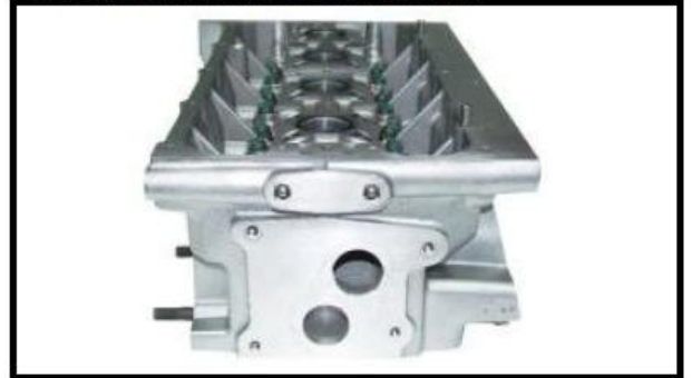
C8-6) Bare cylinderhead seen from flywheel side
