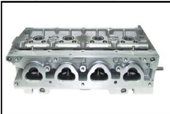
C8-3) Bare cylinderhead seen from intake side
