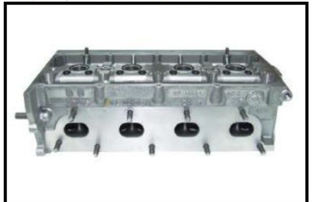
C8-4) Bare cylinderhead seen from exhaust side
