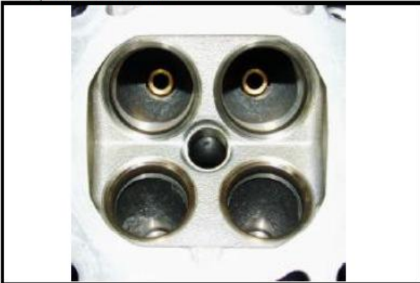
C8-7) Combustion chamber
